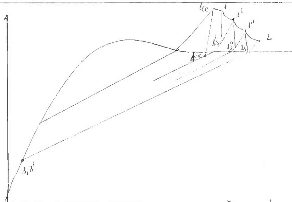
$$\eta_{\text{sil.}}^{\text{efektyn}} = \frac{\dot{m}_{le} + (\dot{m} - \dot{m}_1) \cdot le' + (m - \dot{m}_1' - \dot{m}_2') \cdot le''}{\dot{m}_{\text{par}} \cdot N_D}$$
