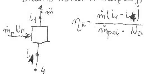
$$\eta_k = \frac{\dot{m}(i_1 - i_4)}{\dot{m}_{pump} \cdot N_D}$$
